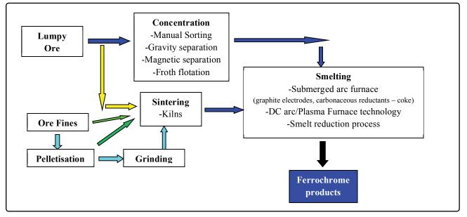
FIGURE 43: TECHNOLOGIES USED IN FERROCHROME PRODUCTION
