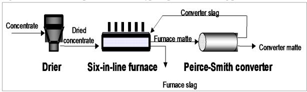
Figure 17: Schematic representation of a typical platinum smelting process
