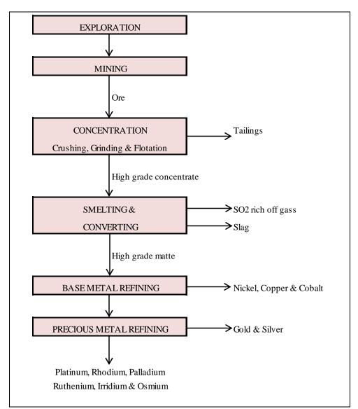
Figure 5: Schematic Flow diagram for the beneficiation of PGM's
